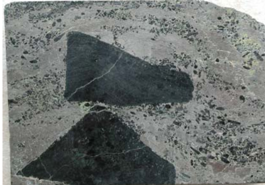
Selected photos of mineralization the Aguablanca deposit. Left: Breccia-like ore including fragments of pyroxenite supported by massive sulphides. The sulphides hosted mm-sized crystals of another pyroxene with equivalent composition. Size sample: 10 cm. Right: Gabbro-norite with disseminated mineralization
